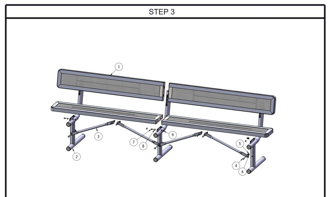
Attach the 29-1/2" Braces to the 940 legs as shown using specified hardware.
