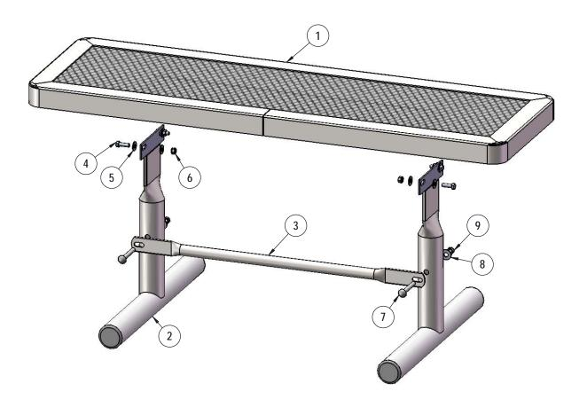
Attach the 29-1/2" Brace to the legs as shown using specified hardware.
