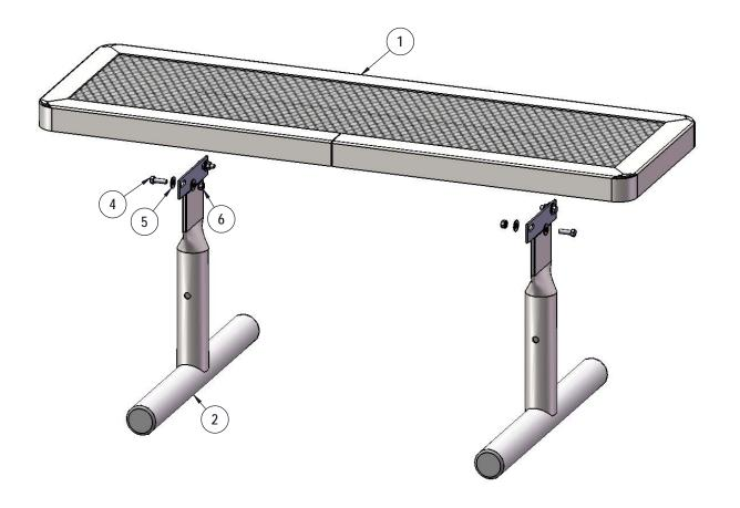
Attach the 4' Expanded Seat to the legs using specified hardware.
