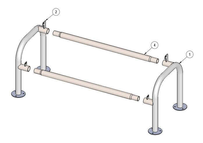
Slide the Spreader Tubes into the Legs.
