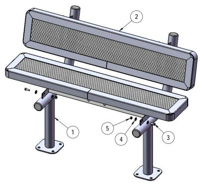
Recommended Surface Mount Hardware: 3/8" x 3-1/2" Concrete Expansion Anchor Bolts (Not Included)
