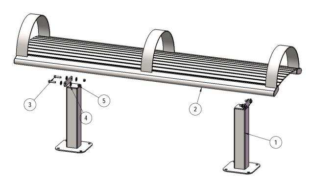
Recommended Surface Mount Hardware: 3/8" x 3-1/2" Concrete Expansion Anchor Bolts (Not Included)
