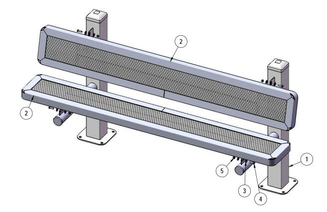
Required Surface Mount Hardware: 3/8" x 3-1/2" Concrete Expansion Anchor Bolts (Not Included)
