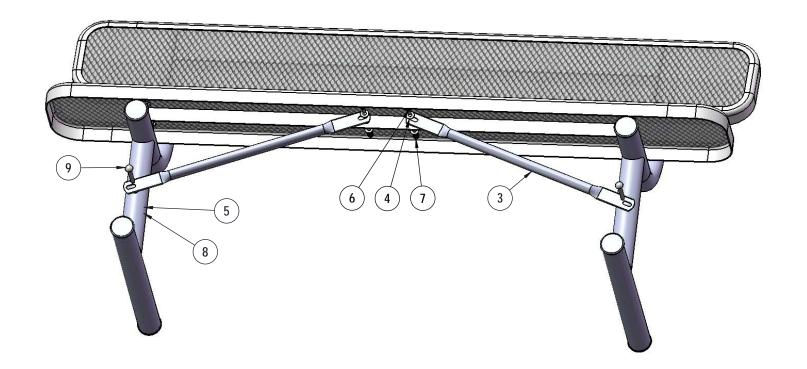
Attach the 26 3/4" bracing as shown using specified hardware.
