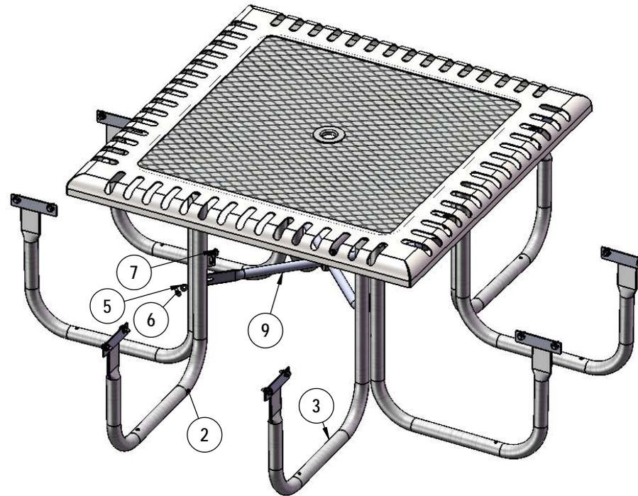
Attach the Cross Brace to the 358 Legs using specified hardware.
