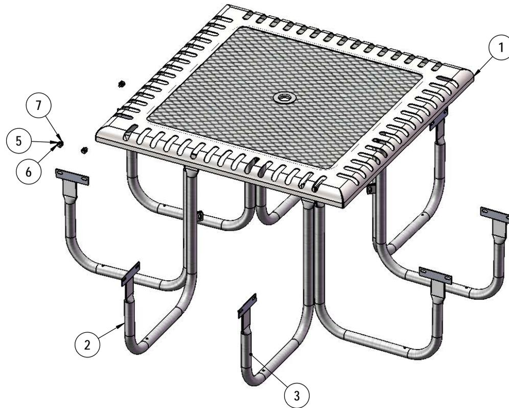
Attach the 358 Legs to the 358 Top using the specified hardware.
