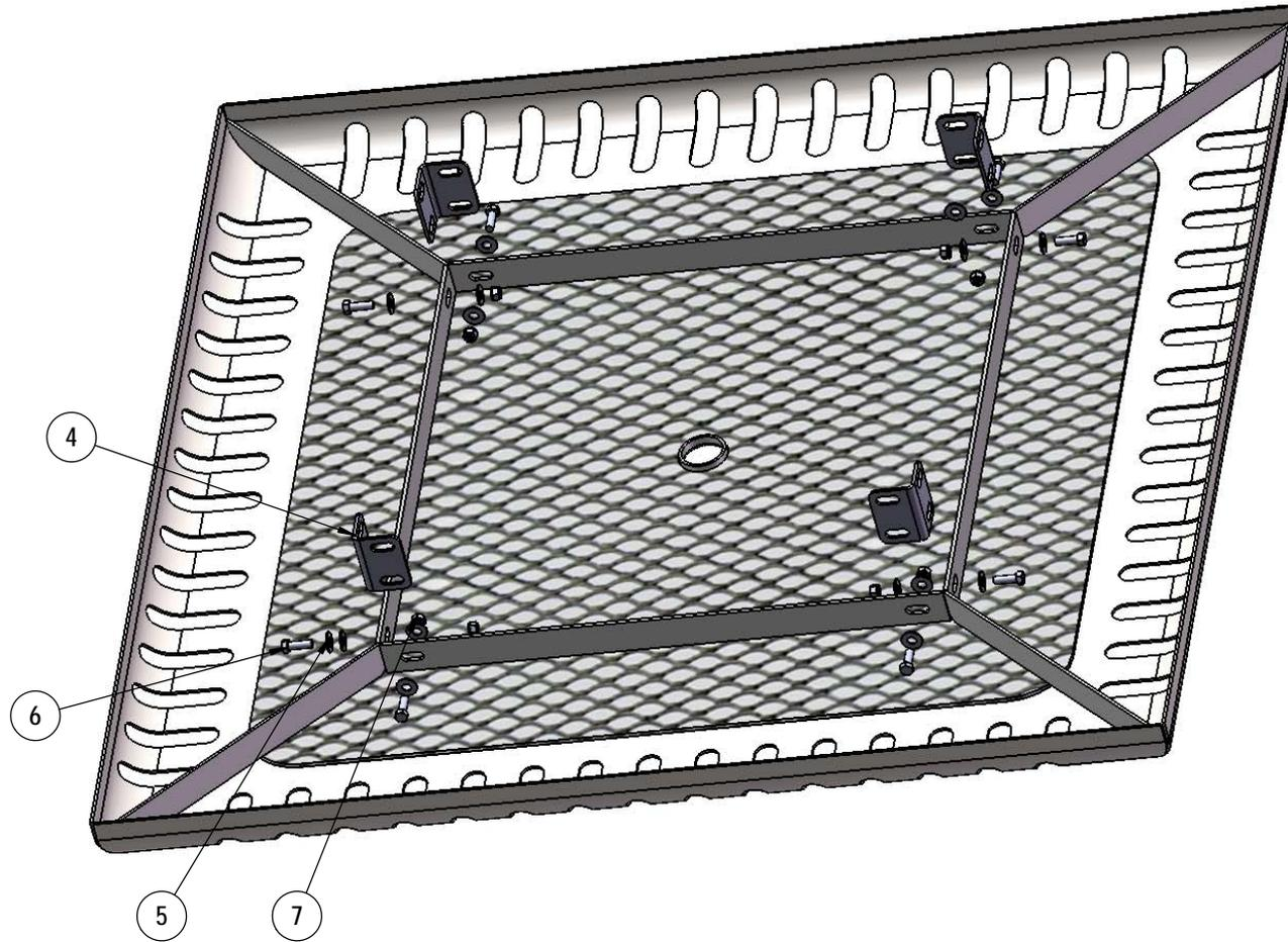
Attach the 358 Extension Tabs to the 358 Top using the specified hardware.
