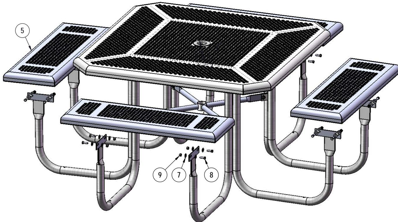
Attach the 3' Seats to the Legs using specified hardware.
