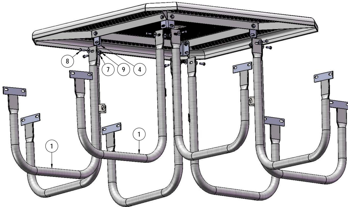
Attach the Legs to the Extension Tabs using specified hardware.
