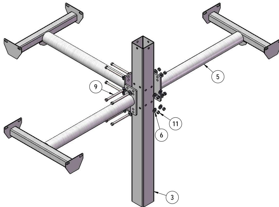
Attach the Arms to the Post using specified hardware.
