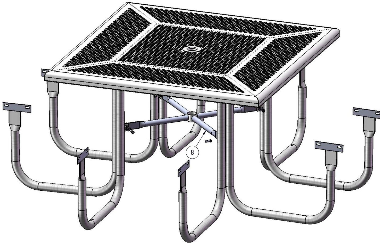
Attach the Crossbrace between the table legs as shown using specified hardware.
