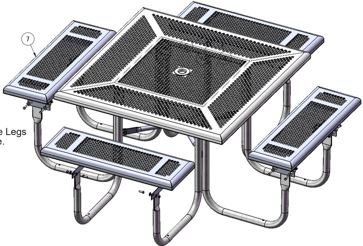
Attach the 3' Seats to the Legs using specified hardware.
