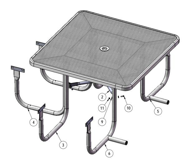
Attach the Crossbrace between the table legs as shown using specified hardware.
