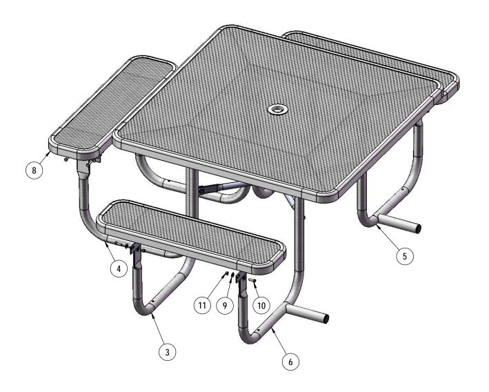
Attach the 3' Seats to the Legs using specified hardware.
