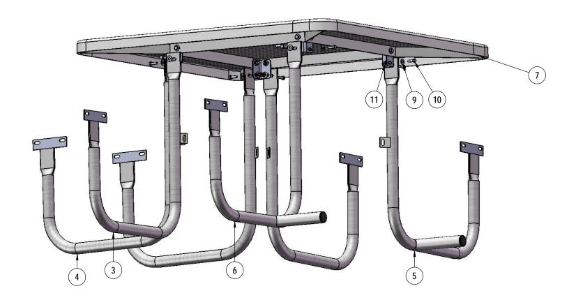
Attach the Legs to the outside of the Extension Tabs using specified hardware.
