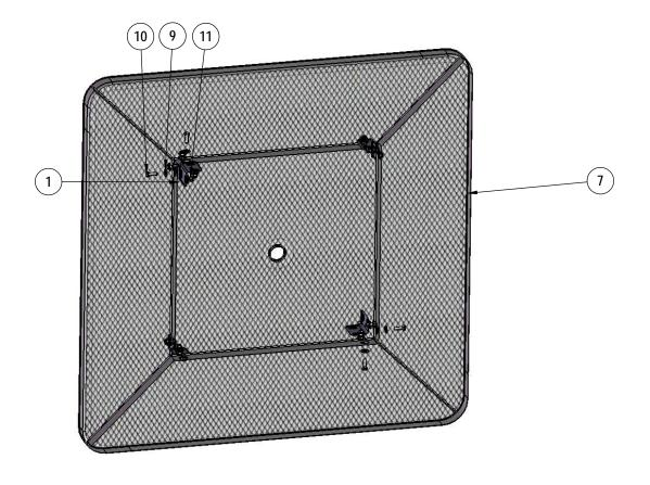
Attach the Extension Tabs to 46" Square Top using specified hardware.
