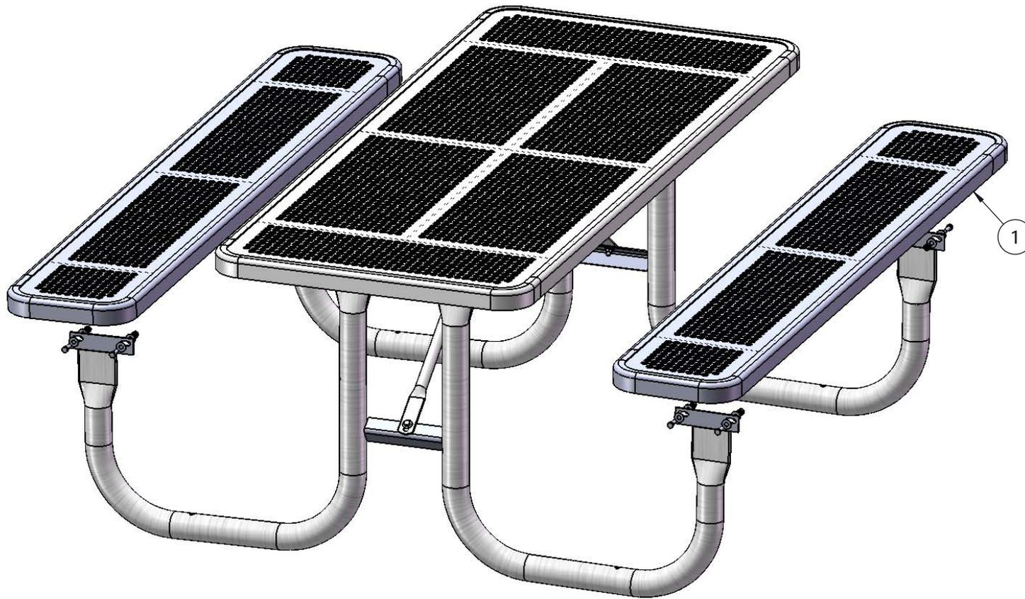
Attach the 6' Punched Seats to the Frames using specified hardware.
