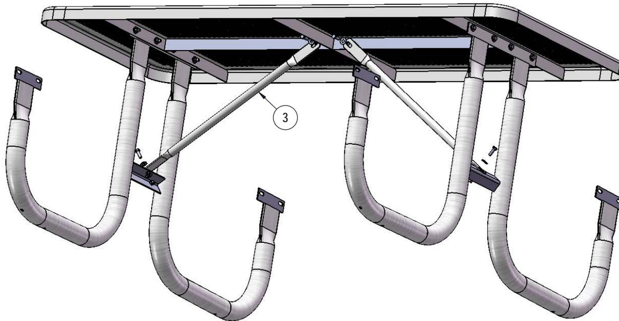
Attach the 29-7/8" Braces to the 6' Punched Top and the Frames as shown using specified hardware.
