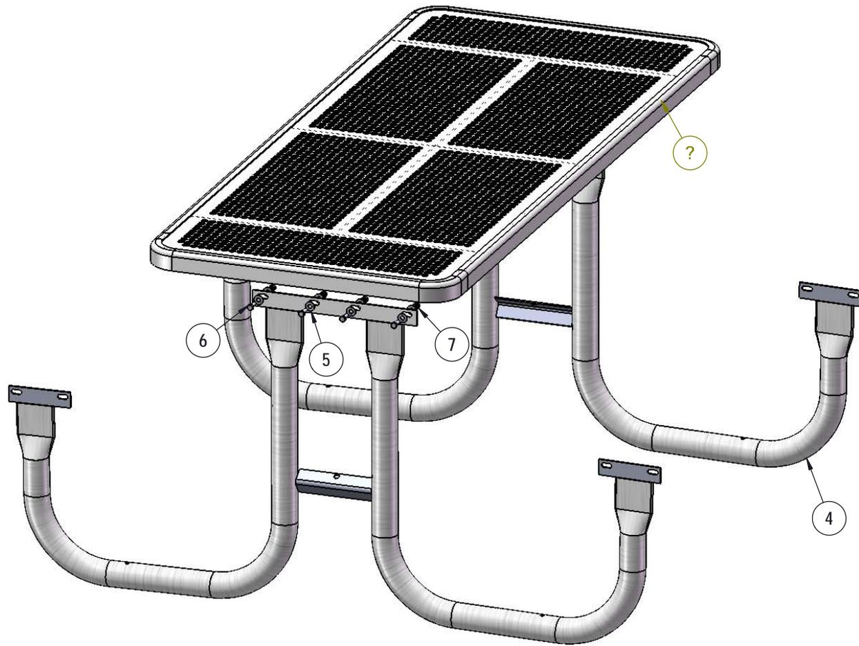
Attach the 6' Punched Top to the Frames using specified hardware.
