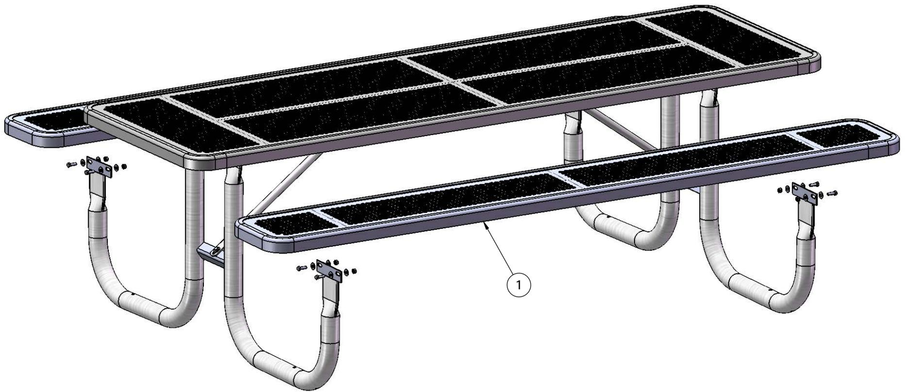
Attach the 29-7/8" Braces to the 8' Punched Top and the Frames as shown using specified hardware.
