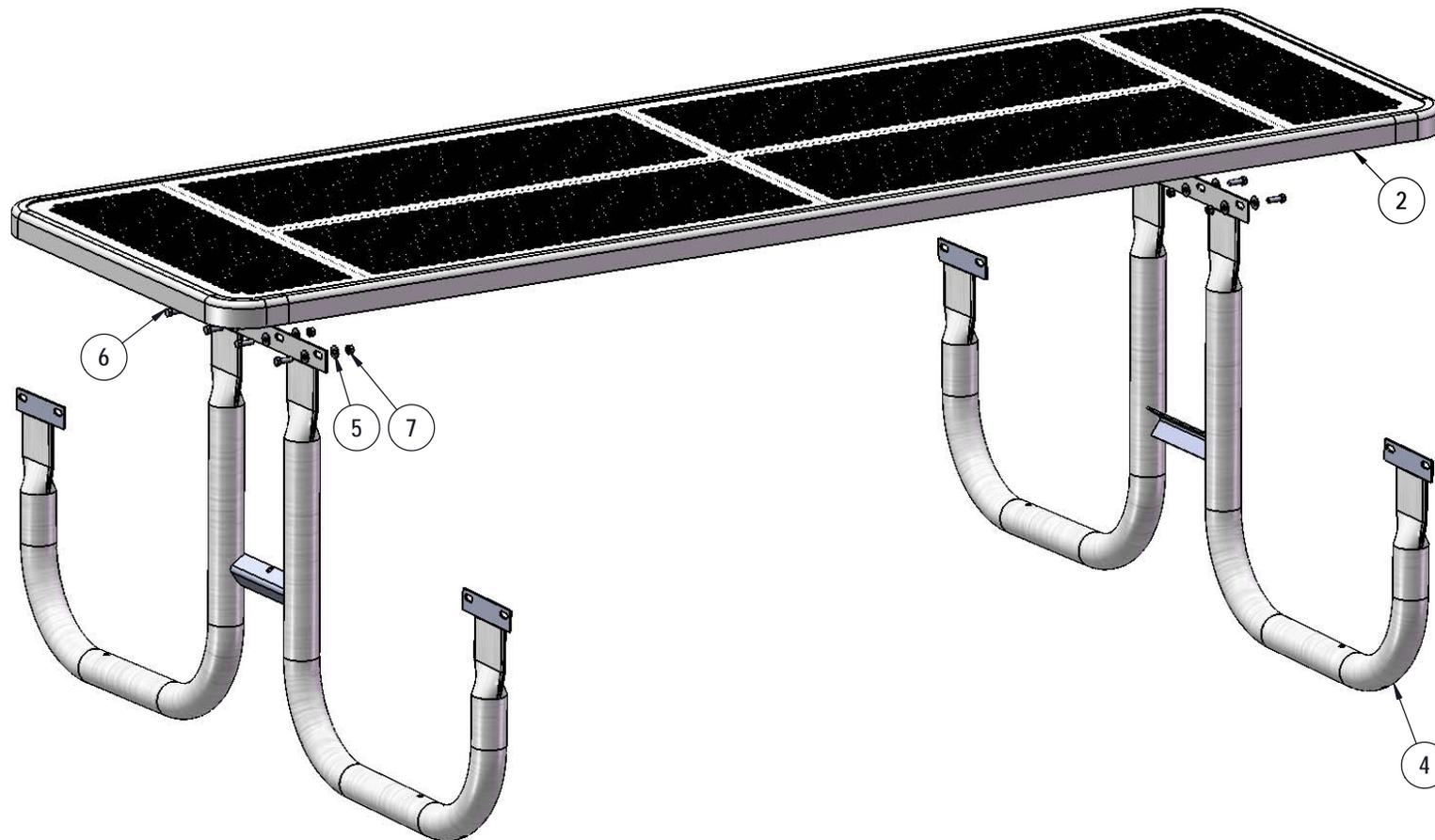
Attach the 8' Punched Top to the Frames using specified hardware.
