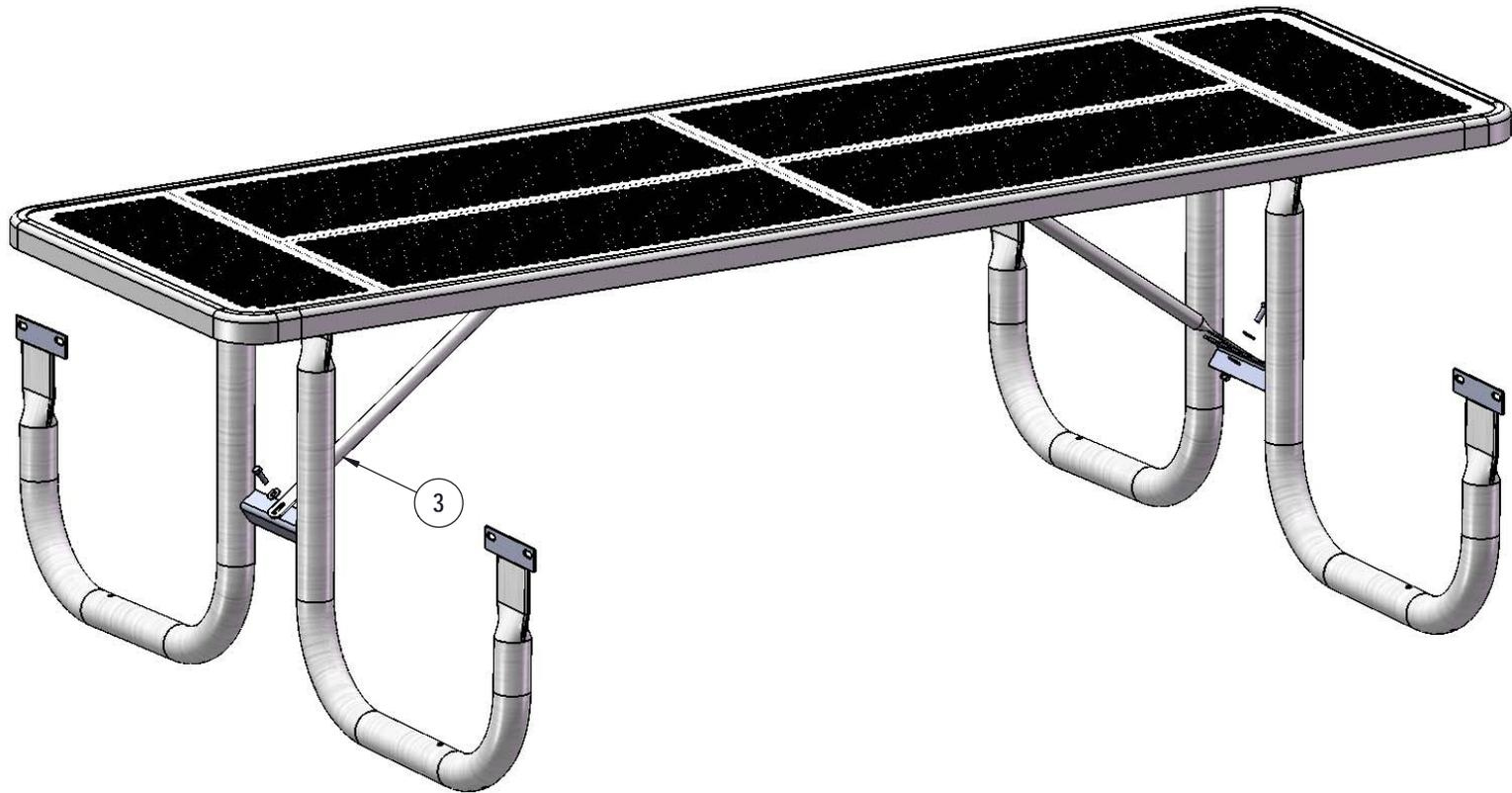
Attach the 29-7/8" Braces to the 8' Punched Top and the Frames as shown using specified hardware.
