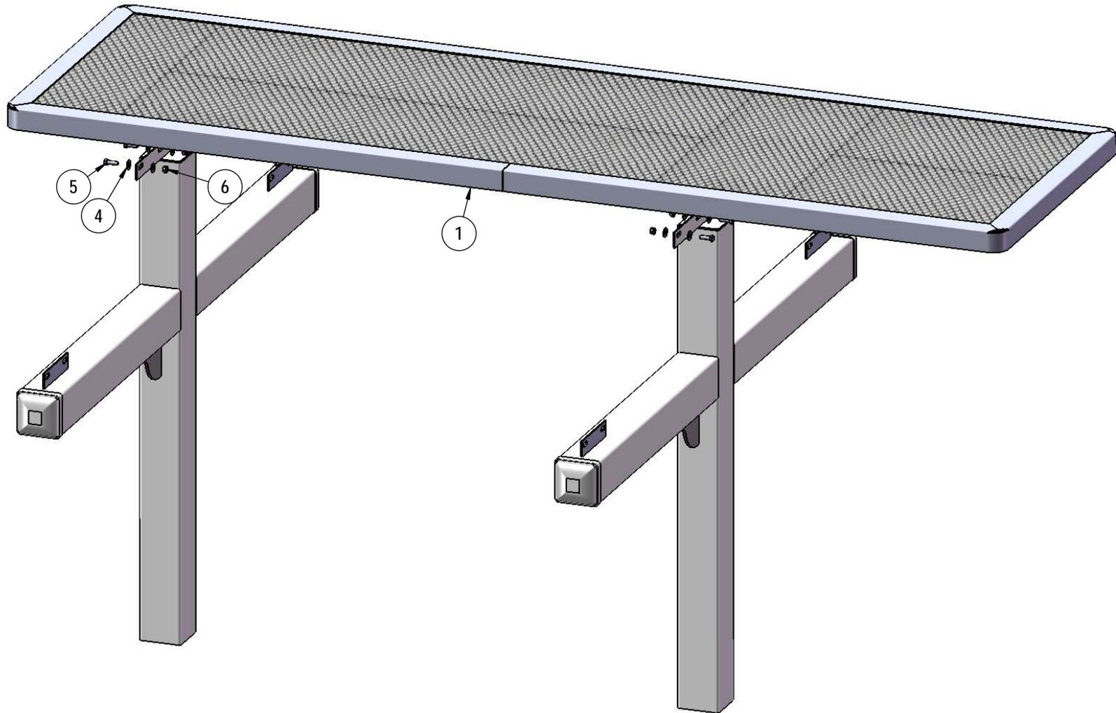
Attach the top to the post assemblies as shown using specified hardware.
