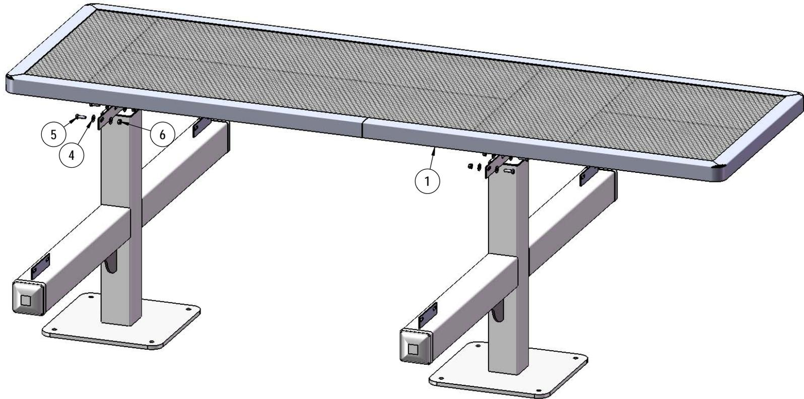
Attach the top to the post assemblies as shown using specified hardware.
