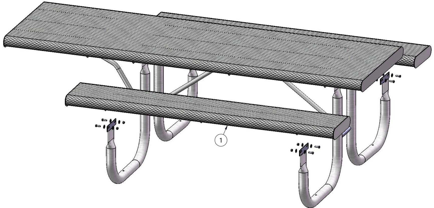
Attach the 6' Vinyl Rolled Seats to the Frames using specified hardware.
