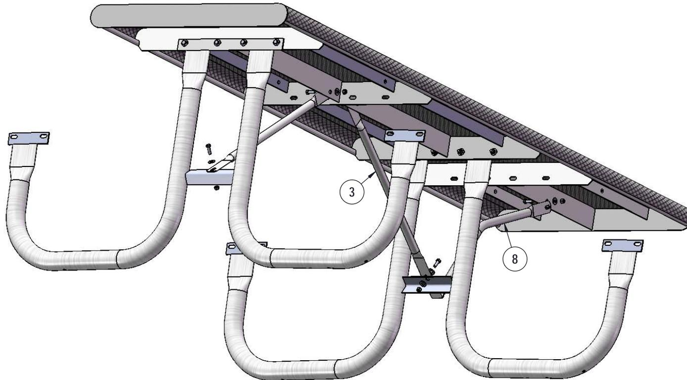
Attach the 29-7/8" Braces to the 8' Vinyl Rolled Top and the Frames as shown using specified hardware.
