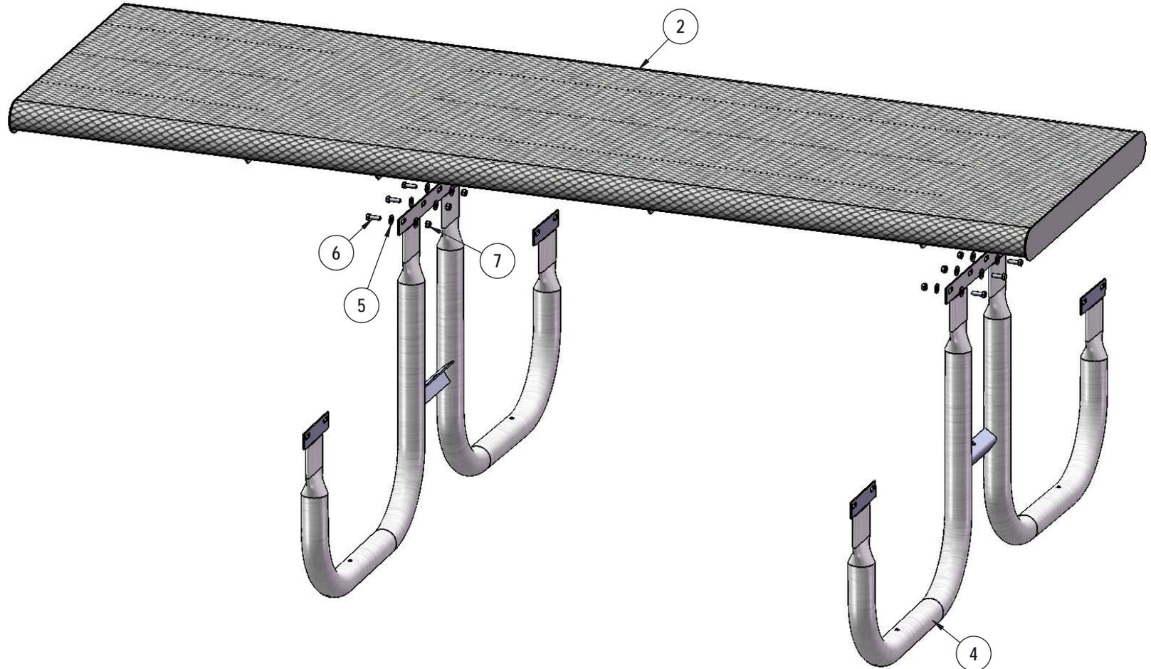
Attach the 8' Vinyl Rolled Top to the Frames using specified hardware.
