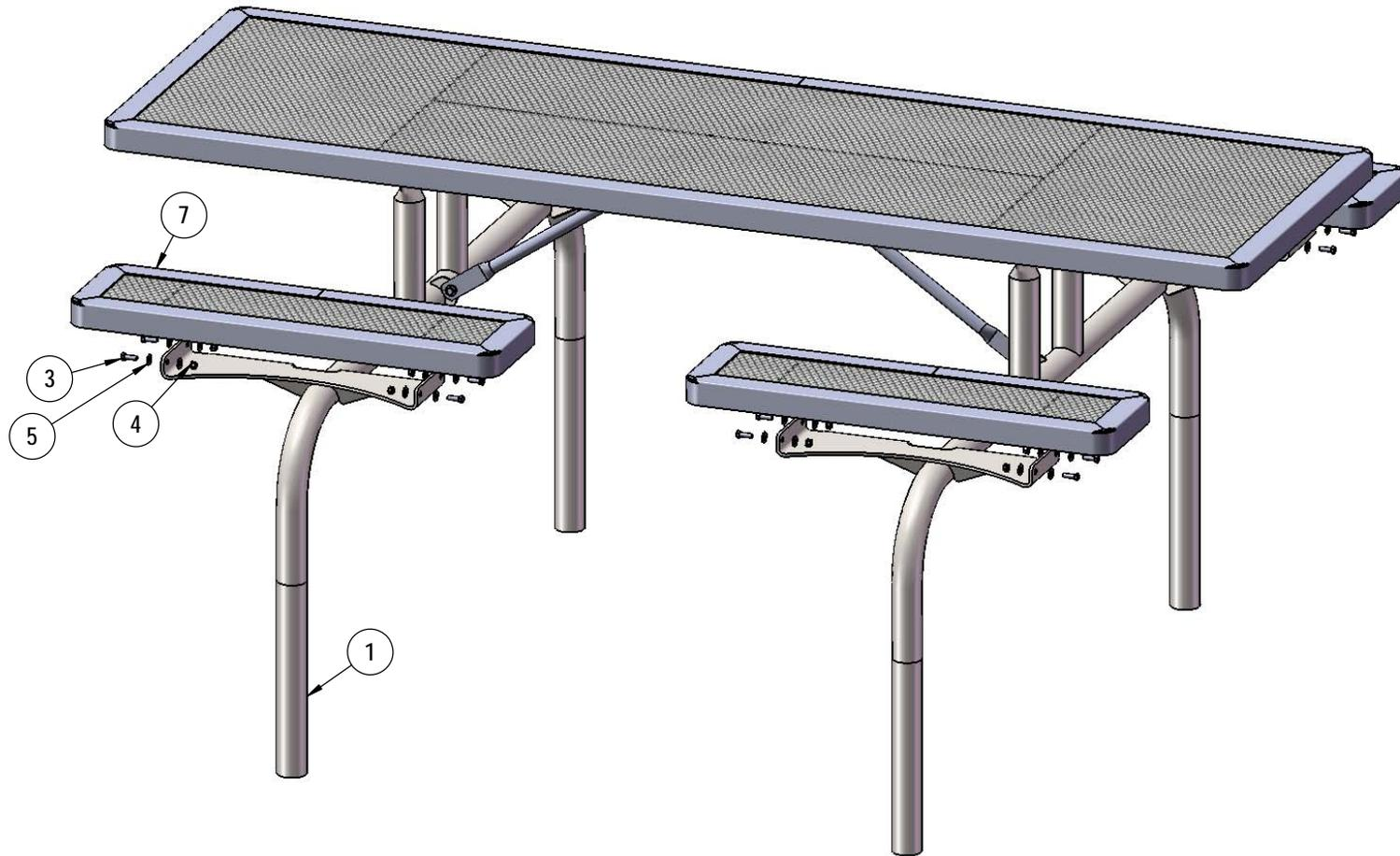
Attach the seats to the legs as shown using specified hardware.
