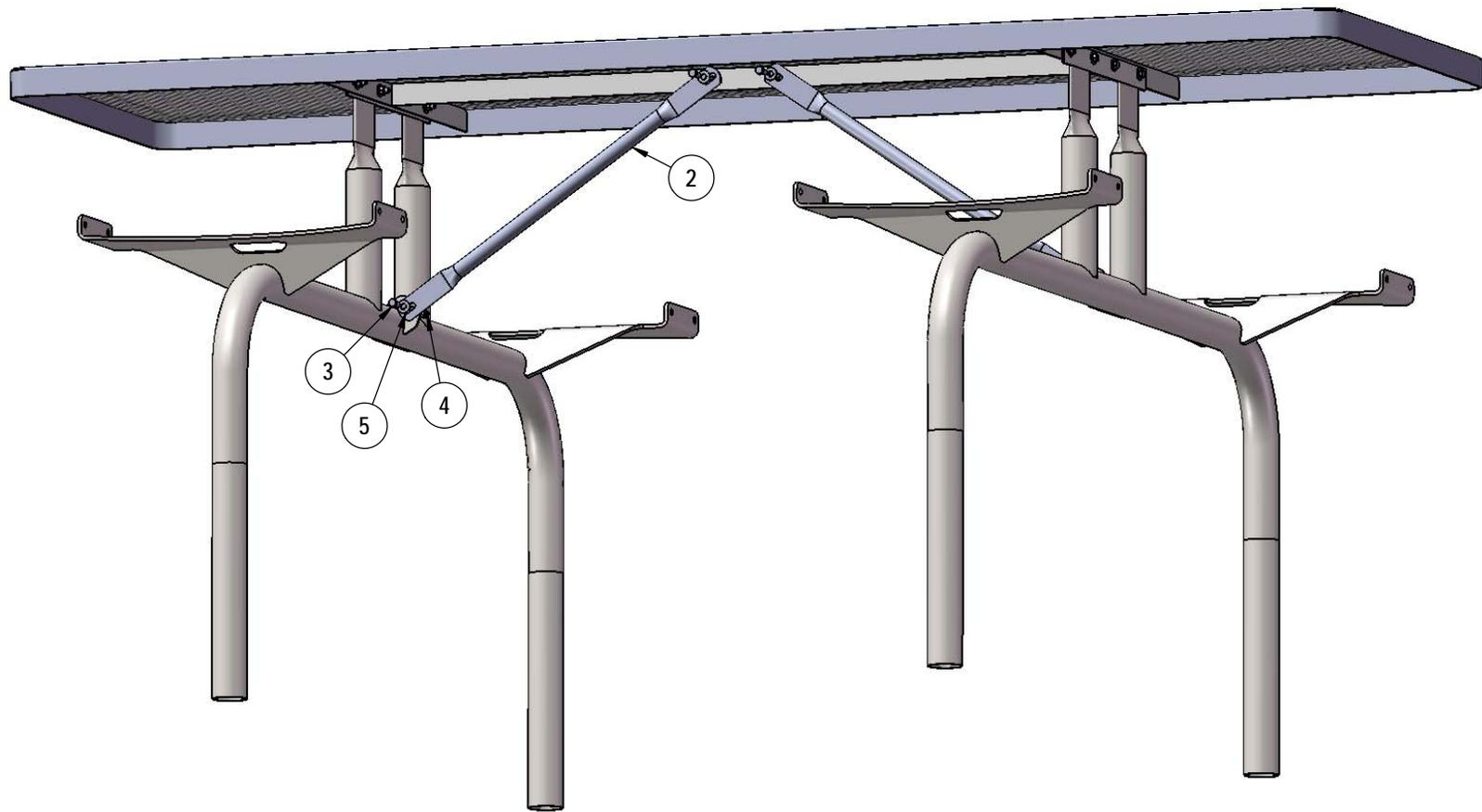
Attach the braces to the legs as shown using specified hardware.
