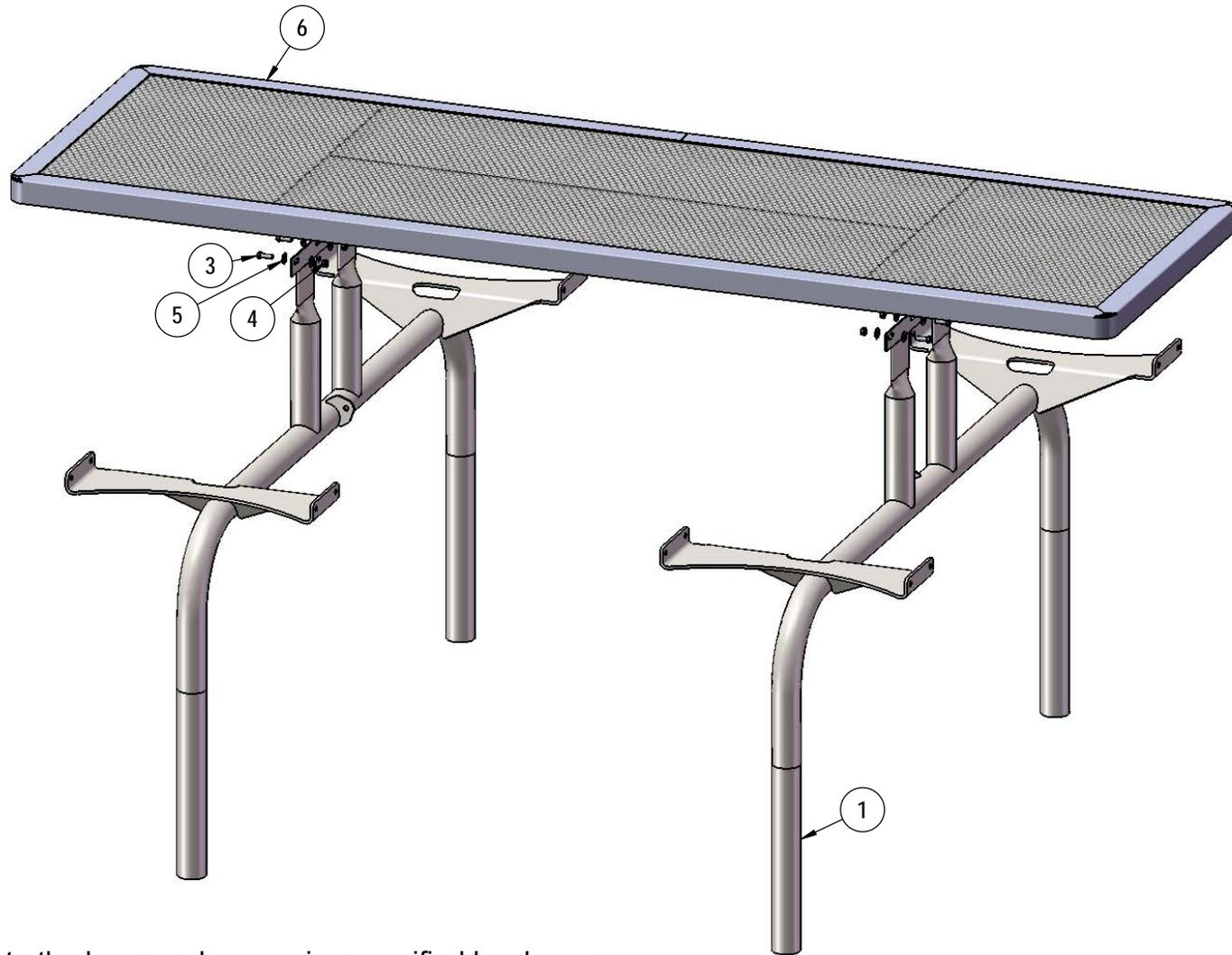
Attach the top to the legs as shown using specified hardware.
