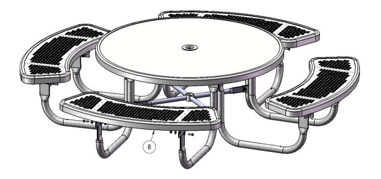
Attach the 3' Round Seats to the Preschool Legs as shown using specified hardware.
