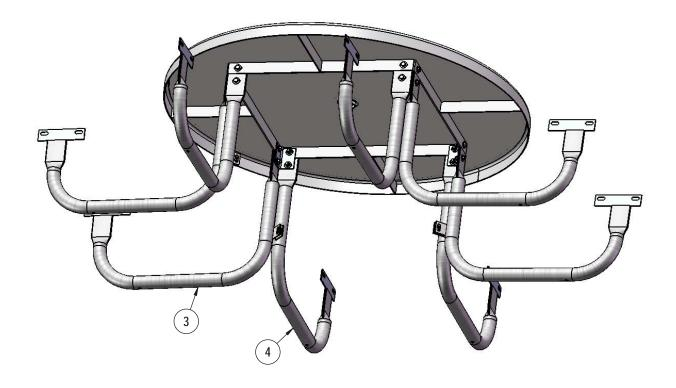
Attach the Preschool Legs to the 358 Extension Tabs as shown using specified hardware.
