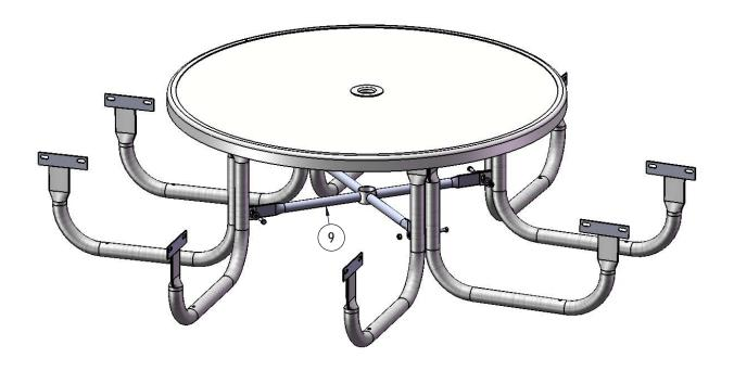
Attach the Cross Brace to the Preschool Legs as shown using specified hardware.
