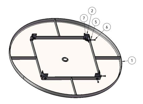
Attach the Extension Tabs to the 46" Round table top as shown using specified hardware.
