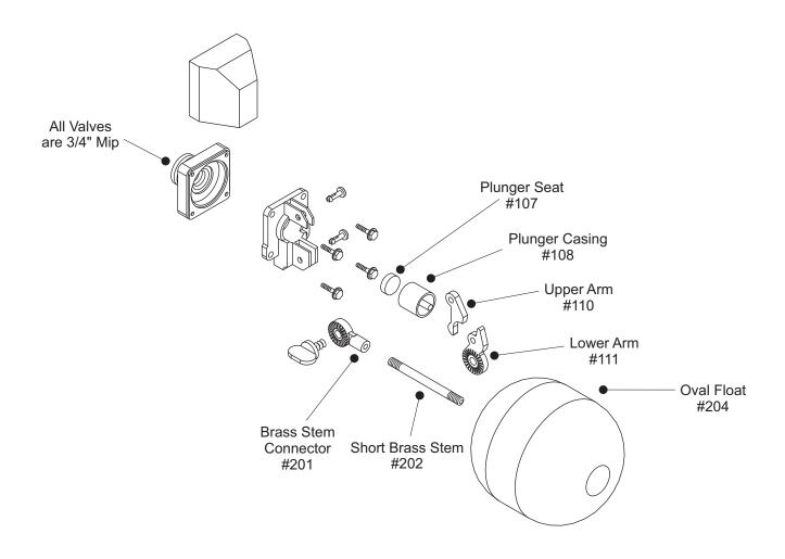
\* Approximate water flow rate of the Float and Valve System with a standard 40-60 psi is 5 - 7 gallons per minute.
