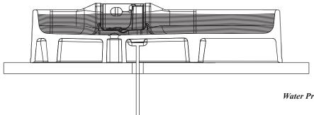
Water Pressure: Please note the valve is appropriate for water pressure up to 55 psi.
